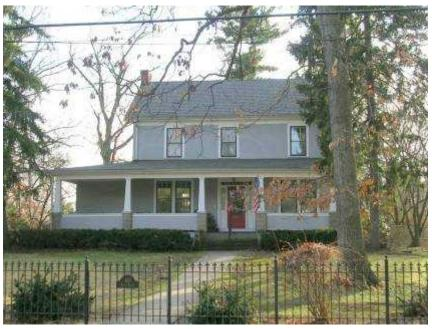
Low eave lines used to reduce scale.
